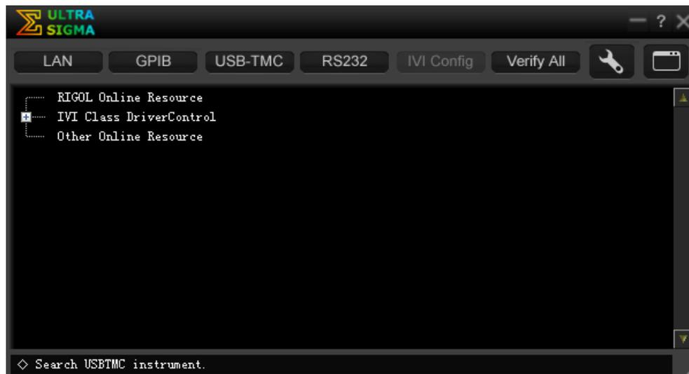
Now please connect your Rigol Instrument thru USB to your computer. Windows will find a new USB Device and start “installing” the driver. After finishing this instrument will appear in your Ultra Sigma Window as follows:
